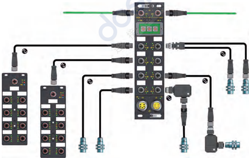
I/O-link连接技术示意图 Schematic diagram of I/O-link connection technology
